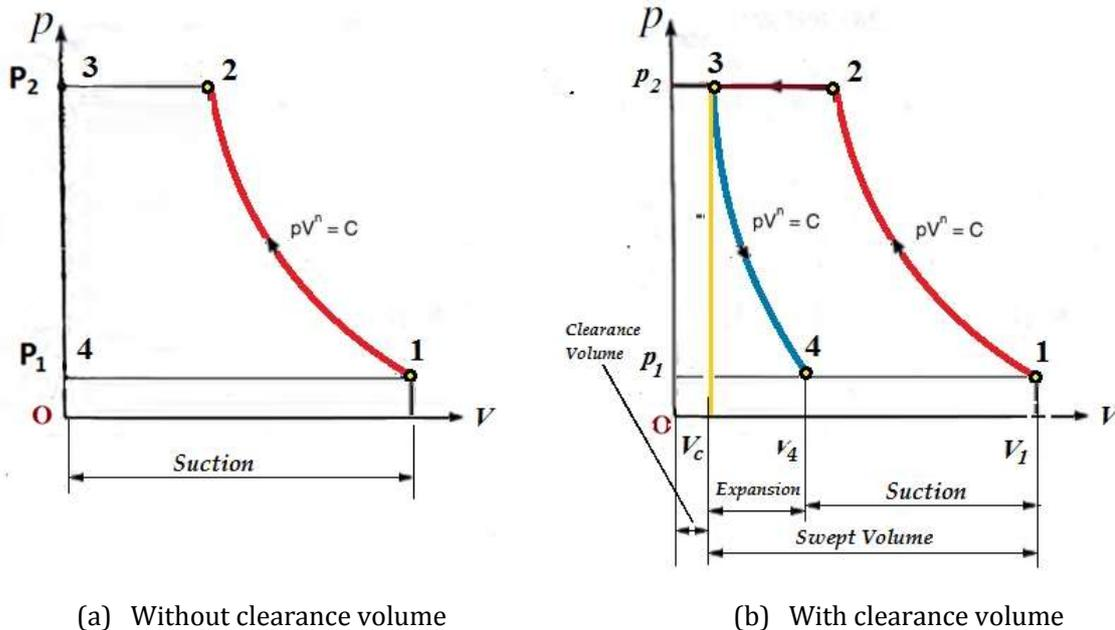
Figure 8, Single stage polytropic compression cycle.
