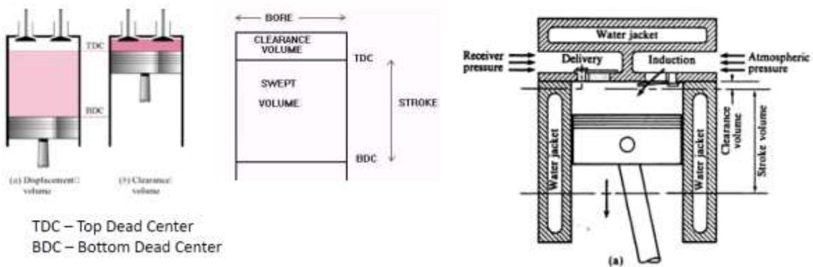
Figure 5: Constructional details of a single acting reciprocating air compressor.
