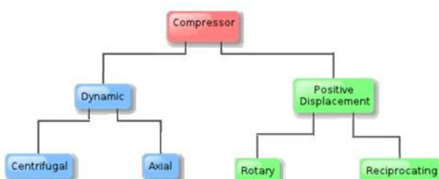
Figure 2: Types of Compressors.
