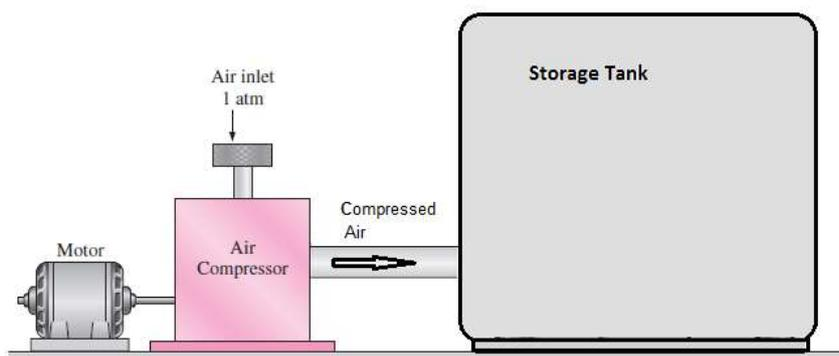
**Figure 1:** Schematic diagram of an Air Compressor unit.
